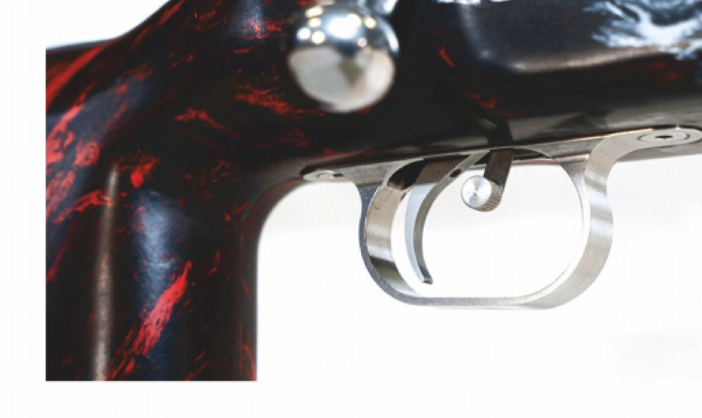
Because the action doesn't have a slot machined for a safety, bottom safeties, such as the one on this Jewell HVRSBR trigger, are a must.
